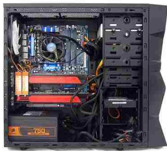
(a) A side view of a personal computer system including a motherboard, graphics card, and power supply connected by physical wires [3].
